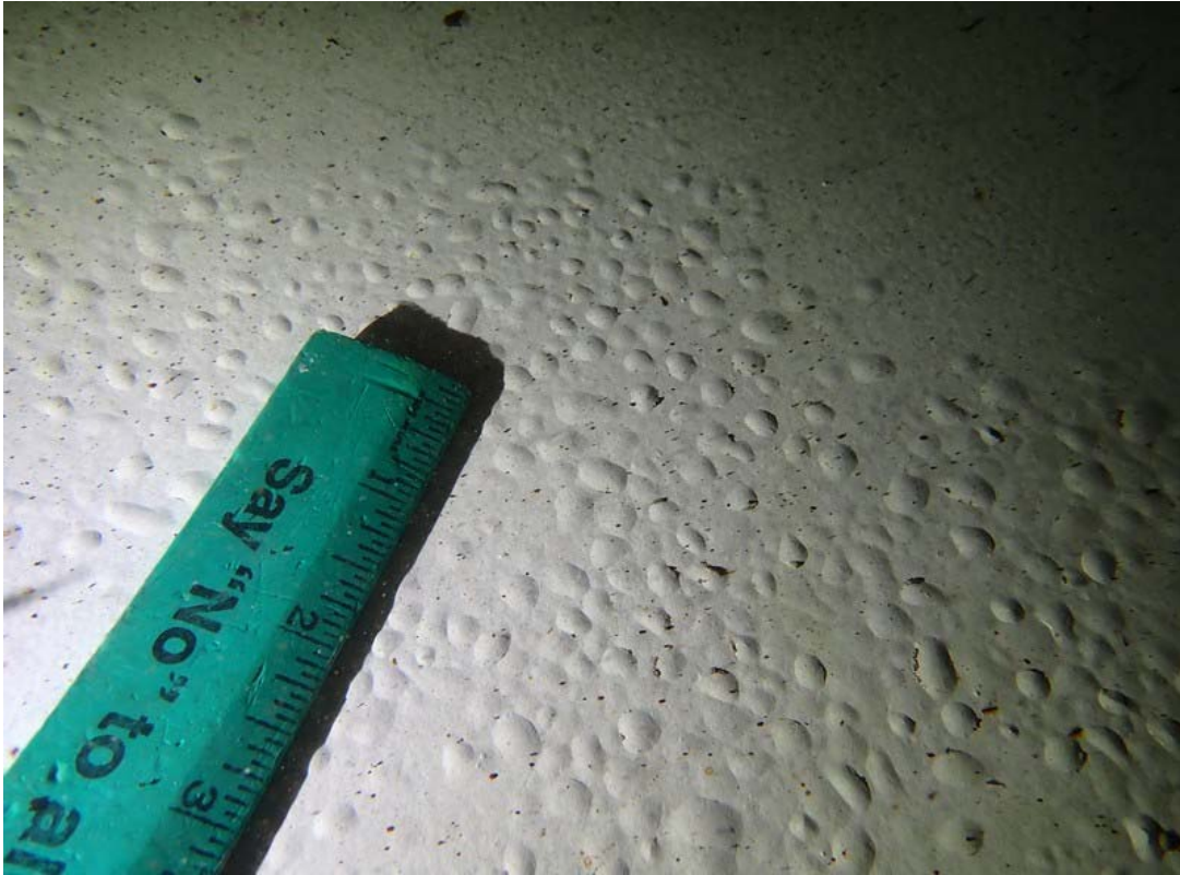
Close view of the interior bottom at an area with a dense pattern of small unbroken blisters. Blisters like this are not uncommon. Unbroken blisters usually do not allow significant corrosion.
